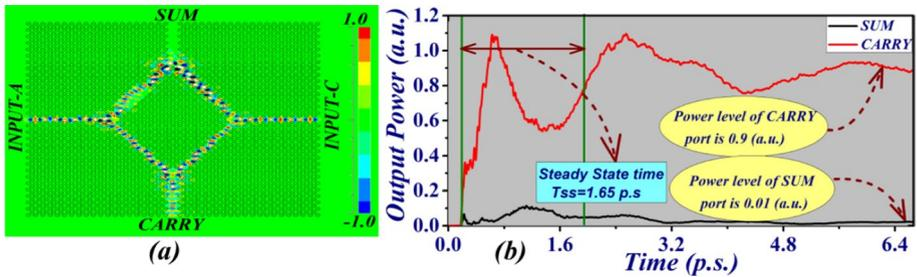
Fig. 5 a Field distribution b time evolving graph, for logic condition ‘11’
