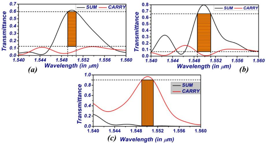
**Fig. 6** Transmittance spectra of the SUM and CARRY ports at input logic states **a** {0,1} **b** {1,0} and **c** {1,1}
