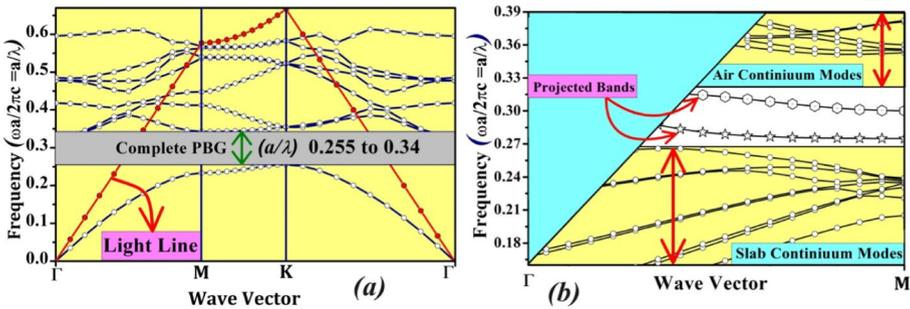
**Fig. 2** **a** Photonic band diagram of non-defect structure **b** projected band diagram of defect structure
