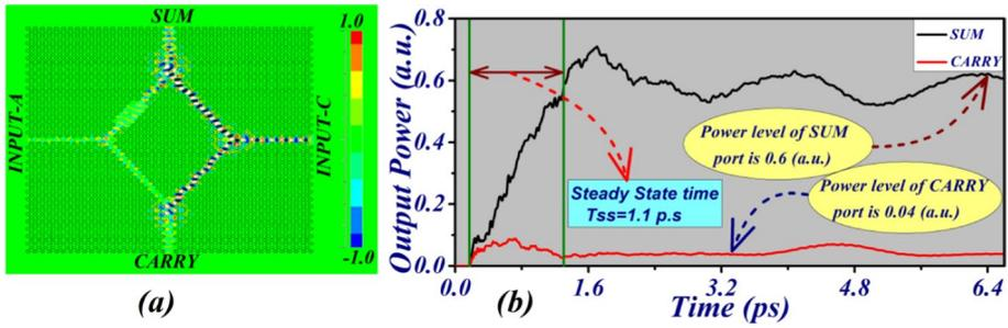
Fig. 4 a Field distribution b time evolving graph, for logic condition ‘10’
